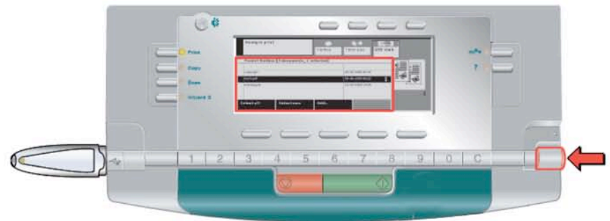
4. Use the scroll wheel to select the document you want to print.
